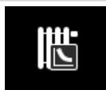
The curve on the control loop icon indicates **weather-dependant regulation**. Weather-dependant regulation of tap water and pool control loops is not possible.
