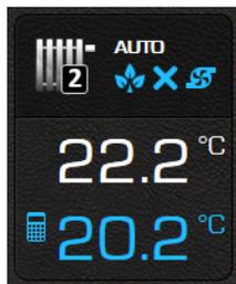
Operation, status and temperature for all control loops present in the system are displayed.
