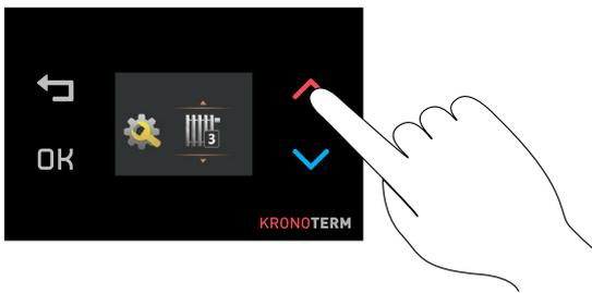
Set the desired heating circuit with the and buttons. Press OK to confirm settings. The control panel confirms valid settings with a multi-tone beep.
