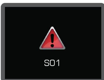
**S01** – Data connection error between spatial corrector and heat pump. Check if the data cable is correctly connected to the connector on the heat pump. After the cause for the error is resolved, the error is automatically confirmed.
