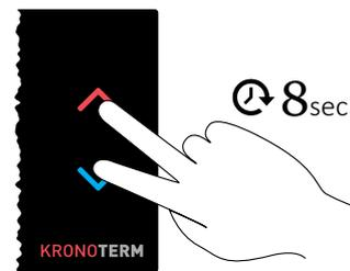
The menu "Setup of control loop" can be accessed only during the first minute of reconnecting the control panel, by holding the and buttons for 8 seconds.
